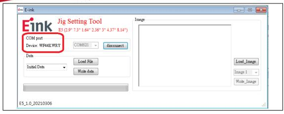
\* After Initial Data are updated, you should press "disconnect" and un-plug/plug Mini USB to restart the kit. If update is successful, the device name will show up
