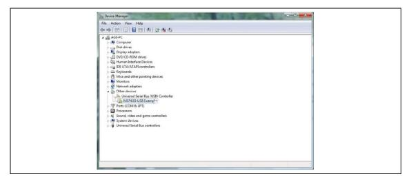
To install the device driver for **MSP430-USB Example**, double click on the device to bring up the device Window. Click on "Update Driver" and select the file "HULK-USB-Driver.inf".
